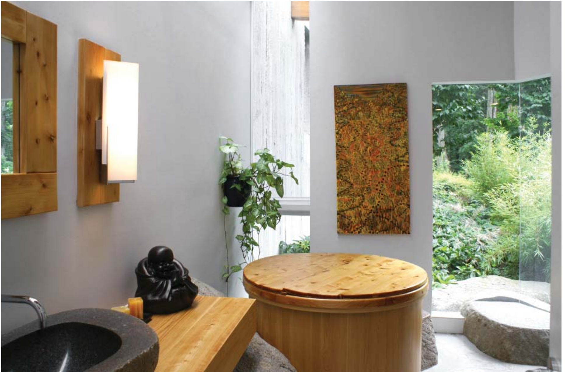
4. BATH- Invisible trim on glass allows wall to continue to outside. Butted glass window shown. Carved granite sink shown.
